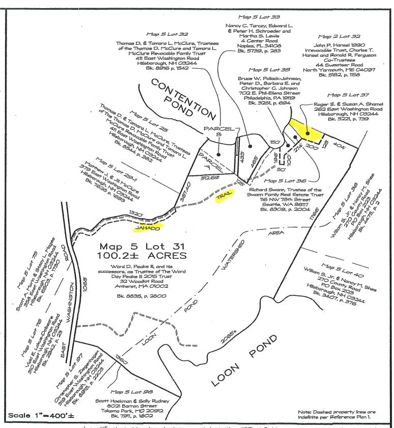
I certify that this plan depicts a total station/EDM field survey made on the ground of Map 5 Lot 32 and Parcels A and B with an unadjusted linear misclosure of 1 part In 115,082 and that all monuments shown are in place Date: February 10, 2017
